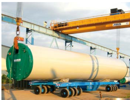
Industrial Lift 80 ton in Germany Used to move Eolic poles sections
