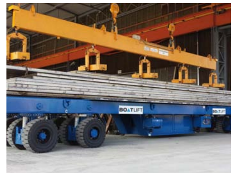
Industrial Lift 130 ton in Germany, Used in ZSB factory and to move steel bridge sections
