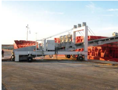
Industrial Lift 20 ton in Italy, Used to move and lift a conveyor belt for ship loading
