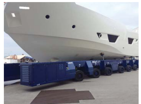
Self-Propelled Cart 240 ton in Italy Used inside the Ferretti CRN Group factory
